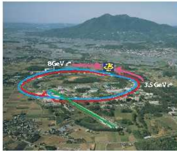
KEKB consists of a linear injector and two 3km-circumference storage rings.
